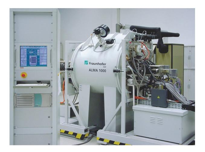
The ALMA evaporation system provides the ability to coat small parts. Credit: Fraunhofer-Gesellschaft
