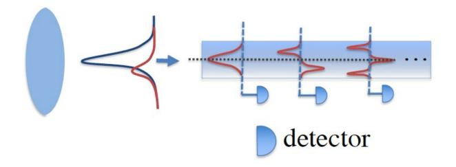
The optimal measurement that achieves the optimal error probabilities, in the limit that the two sources are very close together. It is a multimode waveguide that can be used as a spatial-mode sorter. Photon counting is performed at the output. Credit: Huang & Lupo.
