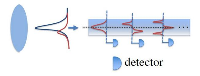
The optimal measurement that achieves the optimal error probabilities, in the limit that the two sources are very close together. It is a multimode waveguide that can be used as a spatial-mode sorter. Photon counting is performed at the output. Credit: Huang & Lupo.
