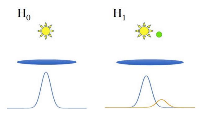
An optical imaging system (modeled as a thin lens) is used to discriminate between two hypotheses. Hypothesis H0: only the star is present. Hypothesis H1: there is a star-planet system present, where the planet has much weaker intensity compared to the star. Credit: Huang & Lupo.
