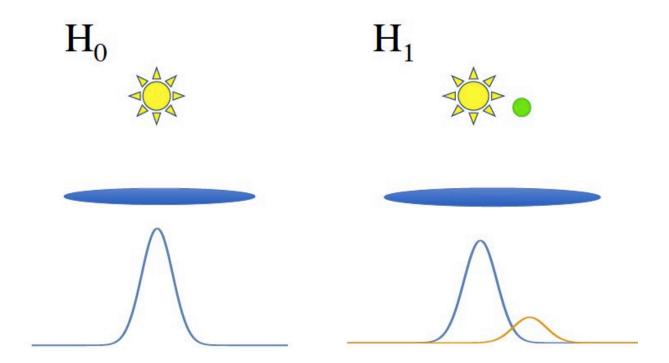
An optical imaging system (modeled as a thin lens) is used to discriminate between two hypotheses. Hypothesis H0: only the star is present. Hypothesis H1: there is a star-planet system present, where the planet has much weaker intensity compared to the star. Credit: Huang & Lupo.
