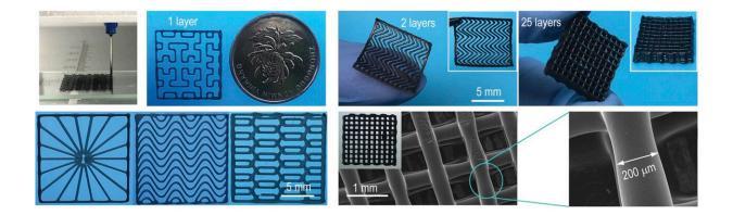
3D printing of SHARK based sensors with predefined shape and microstructures. Credit: Science China Press
