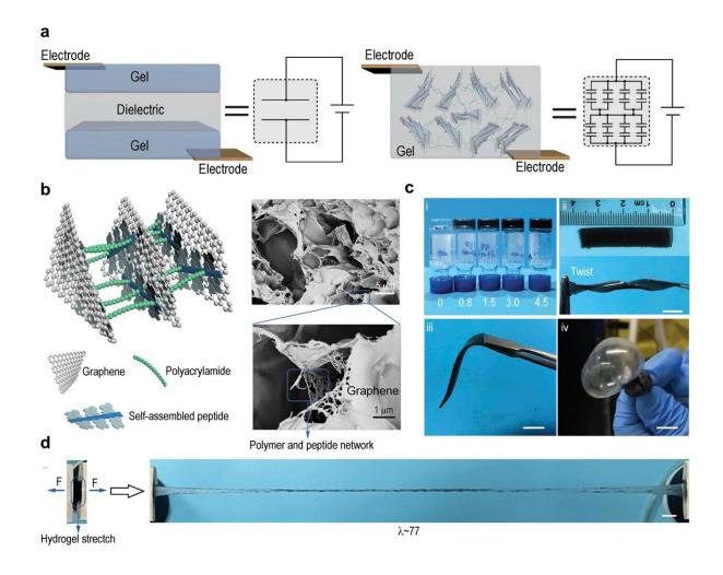
a) Design of SHARK; b) Microstructures of SHARK c-d) Ductility and stretchability of SHARK. Credit: Science China Press
