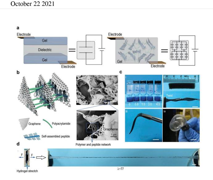
a) Design of SHARK; b) Microstructures of SHARK c-d) Ductility and stretchability of SHARK. Credit: Science China Press
