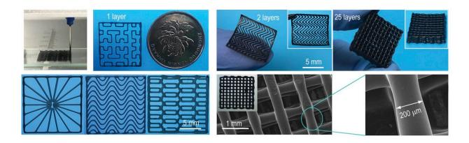
3D printing of SHARK based sensors with predefined shape and microstructures. Credit: Science China Press
