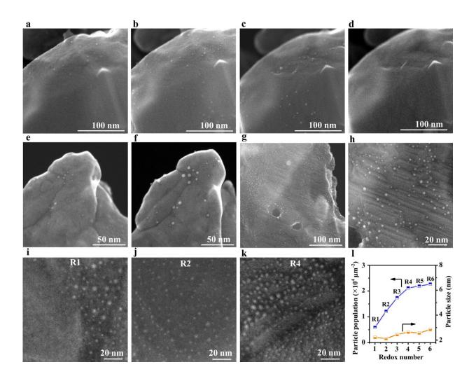
Fig. 1: Morphological study of the SFRuM catalysts. In situ secondary electron (SE)-STEM images of SFRuM after reduction at 800 °C for ~15 min (a), after reduction at 800 °C for ~30 min (b), after reoxidation at 800 °C for ~30 min (c),
