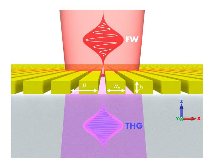
A metasurface made of arsenic trisulfide nanowires (yellow) transmit an incoming near-infrared frequency (red) as well as its third harmonic ultraviolet frequency (violet), which would normally be absorbed by the material. Credit: Duke University
