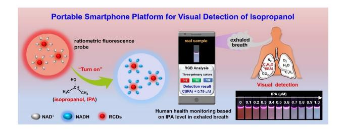
Schematic diagram of the detection of isopropanol in exhaled air by a smartphone fluorescence sensor platform. Credit: YANG Fan
