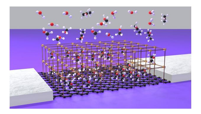
The sensor unit consists of a graphene field effect transistor on which a surfacemounted metal-organic framework is grown. Credit: Sandeep Kumar, KIT
