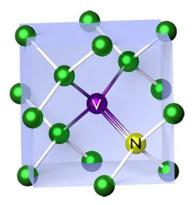
During diamond's formation, replacement of a carbon atom (green) with a nitrogen atom (yellow, N) and omitting another to leave a vacancy (purple, V) creates a common defect that has well-defined spin properties. Credit: NIST
