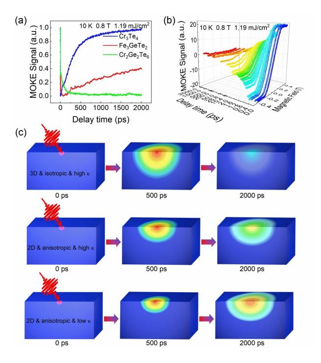
Compared with the other two materials, Cr<sub>2</sub>Ge<sub>2</sub>Te<sub>6</sub> exhibits ultra-long spin relaxation behavior after complete demagnetization. Credit: SUN Tao
