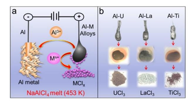
Figure: IAP process. (a) Schematic illustration of the IAP process in NaAlCl4 molten salt electrolyte. (b) Various alloys and corresponding metal chlorides precipitated in the bottom of the crucible by electrolysis with different anodes and final metal chloride products obtained. Credit: IHEP
