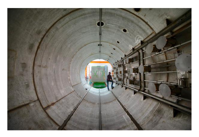
Workers install a component of MicroBooNE's precision detector (called a time projection chamber) into the cylindrical container, or cryostat. Credit: Reidar Hahn, Fermilab.
