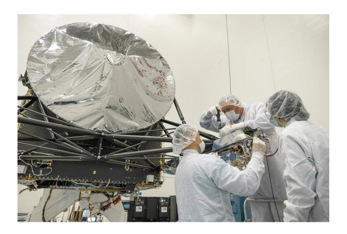
At NASA's Jet Propulsion Laboratory, engineers integrate a gamma ray and neutron spectrometer into the agency's Psyche spacecraft. The instrument will help determine the elements that make up its target, an asteroid also named Psyche. Credit: NASA/JPL-Caltech
