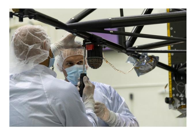
Engineers at NASA's Jet Propulsion Laboratory in Southern California integrate the magnetometer instrument into the agency's Psyche spacecraft on June 28,
