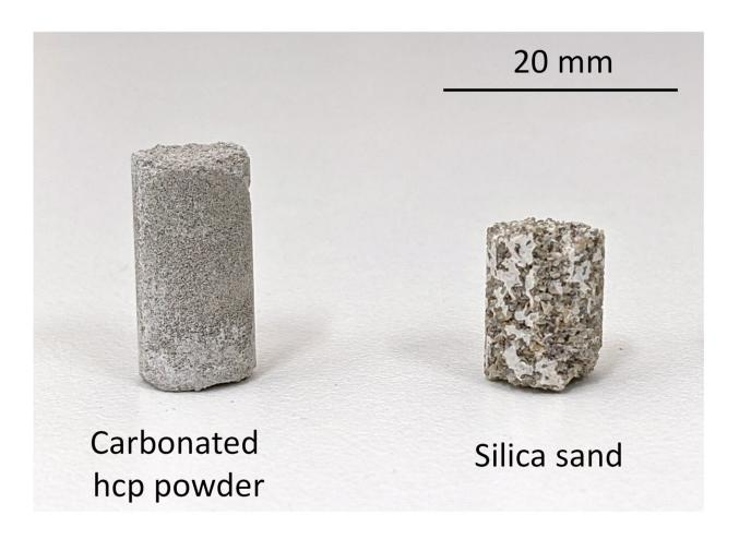
Two samples of calcium carbonate concrete, one using hardened cement paste (left) and the other using silica sand. Both raw materials are common construction and demolition waste products. Credit: Maruyama et al.
