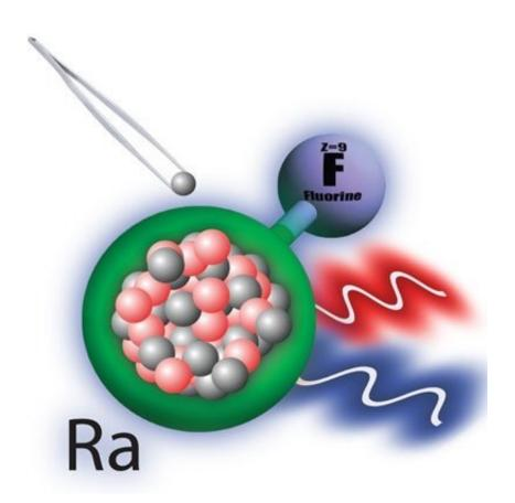
Changing the number of neutrons (grey spheres) in the radium (Ra) nucleus changes the energy levels of the radium monofluoride (RaF) molecule. Small changes can be measured by using different lasers (blue and red wavy lines). Credit: Silviu-Marian Udrescu, Massachusetts Institute of Technology
