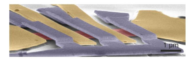
Scanning electron microscope image of a contacted, two-atom-thick, free-floating graphene flake with a free-floating metal bridge hovering above it. Credit: Fabian Geisenhof/Jakob Lenz
