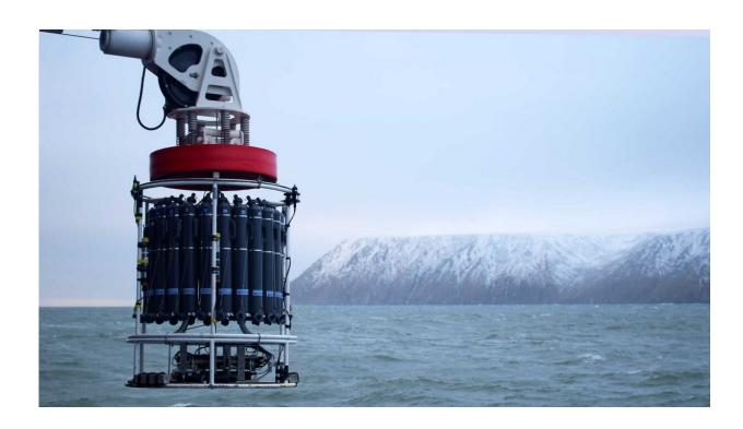
A water sampler known as a conductivity, temperature, depth (CTD) rosette is deployed from the U.S. Coast Guard icebreaker Healy during a 2019 expedition to the Alaskan Arctic Ocean to study the presence of harmful algae and the conditions that promote their growth and spread. Credit: Woods Hole Oceanographic Institution
