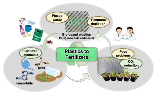
Using the degradation products of PIC as a nitrogen-rich fertilizer closes a sustainable loop that makes bioplastics a much more attractive option for addressing the environmental issues posed by conventional petroleum-based plastics. Credit: Daisuke Aoki from Tokyo Institute of Technology
