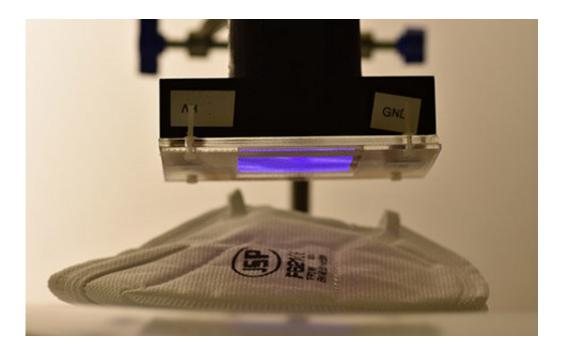
The prototype decontamination system applying cold plasma to sample PPE. Credit: University of Southampton
