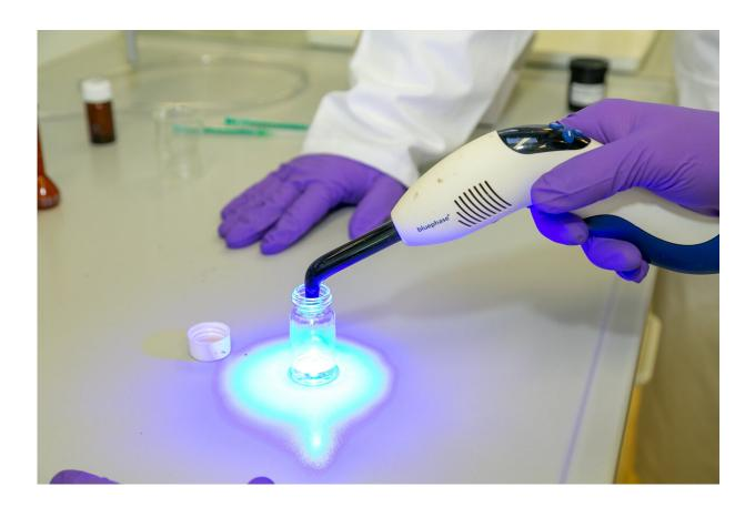
Researchers at Graz University of Technology have developed a new, significantly cheaper production method for germanium-based photoinitiators. This opens up further fields of application beyond the dental sector. Credit: Frankl - TU Graz
