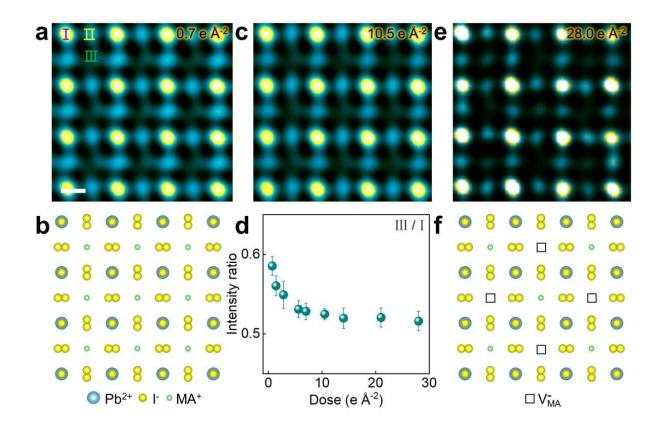
Fig. 1 Atomic-imaging of the loss of MA+ and intermediate phase. Credit: SIAT
