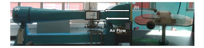
The wind tunnel and scaled model of the overpass. Credit: Alex Ensign
