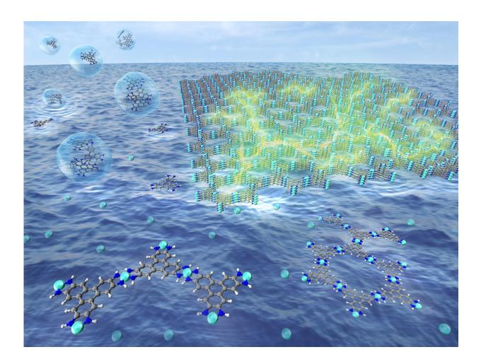
Simple spreading of droplets containing molecular components on the surface of water leads to spontaneous formation of nanostructures with very high electrical conduction. Credit: Rie Makiura, Osaka Prefecture University
