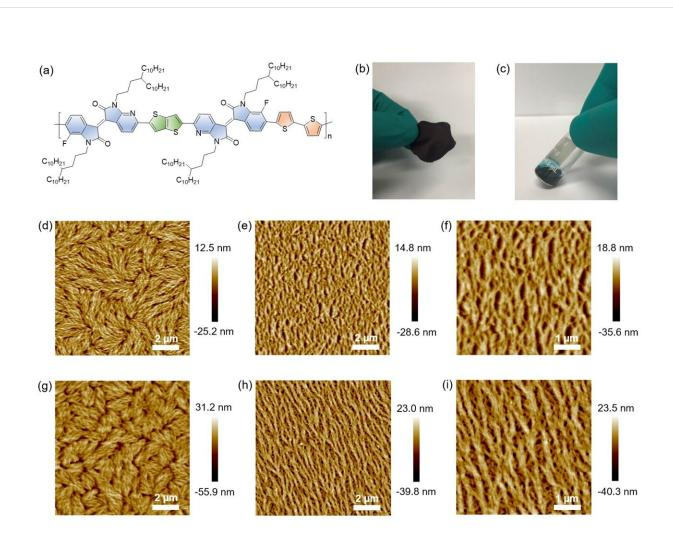
(a) Molecular structure of PITTI-BT. (b) Photograph of PITTI-BT film. (c) Pxylene solution of PITTI-BT. AFM images of the polymer films prepared by (d,g) on-center and (e,f,h,i) off-center SC methods from (d–f) p-xylene or (g–i) o-dichlorobenzene solution. Photo credit: Jie Yang. Credit: Science China Press
