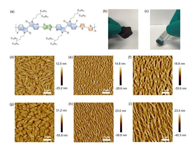
(a) Molecular structure of PITTI-BT. (b) Photograph of PITTI-BT film. (c) P-xylene solution of PITTI-BT. AFM images of the polymer films prepared by (d,g) on-center and (e,f,h,i) off-center SC methods from (d–f) p-xylene or (g–i) o-dichlorobenzene solution. Photo credit: Jie Yang. Credit: Science China Press
