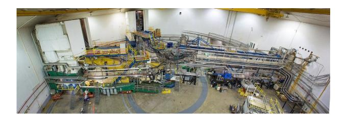
Jefferson Lab Hall A features two High Resolution Spectrometers. Credit: DOE's Jefferson Lab
