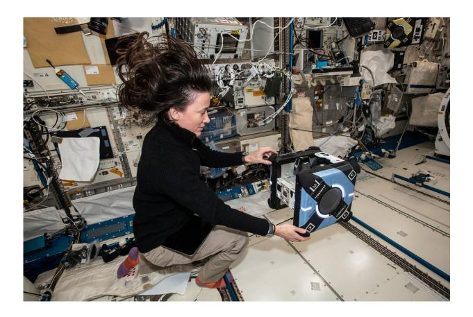
NASA astronaut and Expedition 65 Flight Engineer Megan McArthur sets up an Astrobee robotic free flyer inside the International Space Station's Kibo laboratory module. Credit: NASA
