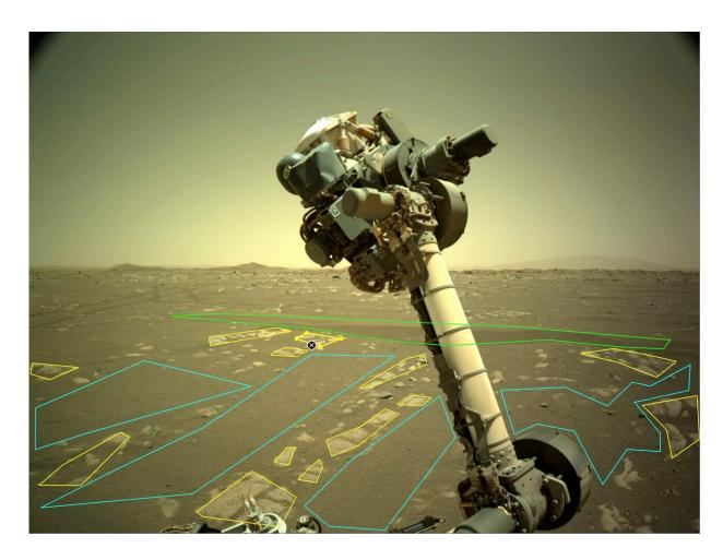
The robotic arm of NASA's Perseverance rover is visible in this image used by the AI4Mars project. Users outline and identify different rock and landscape features to help train an artificial intelligence algorithm that will help improve the capabilities of Mars rovers. Credit: NASA/JPL-Caltech
