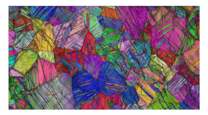
Scientists at Berkeley Lab's Molecular Foundry used an electron microscopy technique called electron backscatter diffraction (EBSD) to image the structure of pure titanium with a nanotwinned structure. Each color represents a unique orientation of the grains. The thin strips reveal the nanotwinned structure produced via a process called cryo-forging. Credit: Andy Minor/Berkeley Lab
