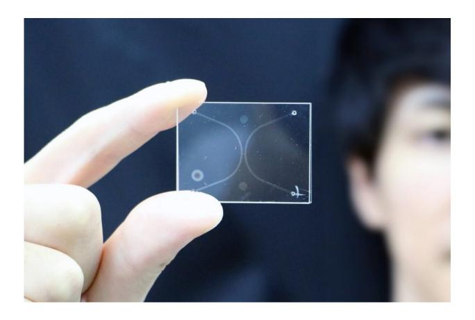
A nanofluidic device enabling fabricating nanoscale gas-liquid interfaces. Credit: Yan Xu, Osaka Prefecture University
