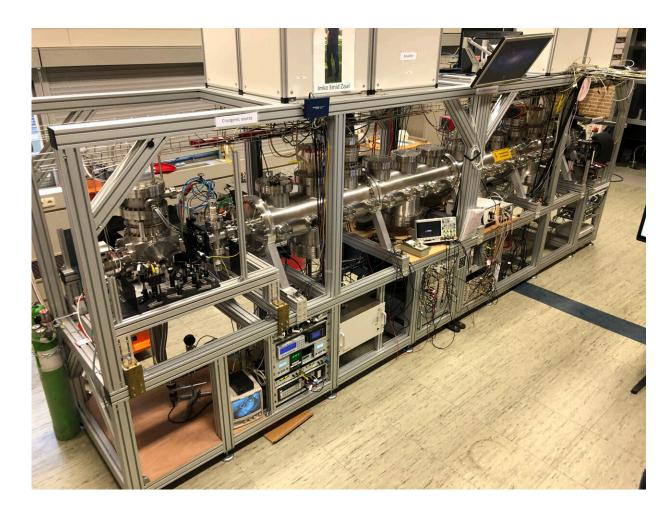
The 4.5-meter long experimental setup. On the left, the chamber in which the strontium fluoride molecules are created. Credit: Steven Hoekstra, University of Groningen
