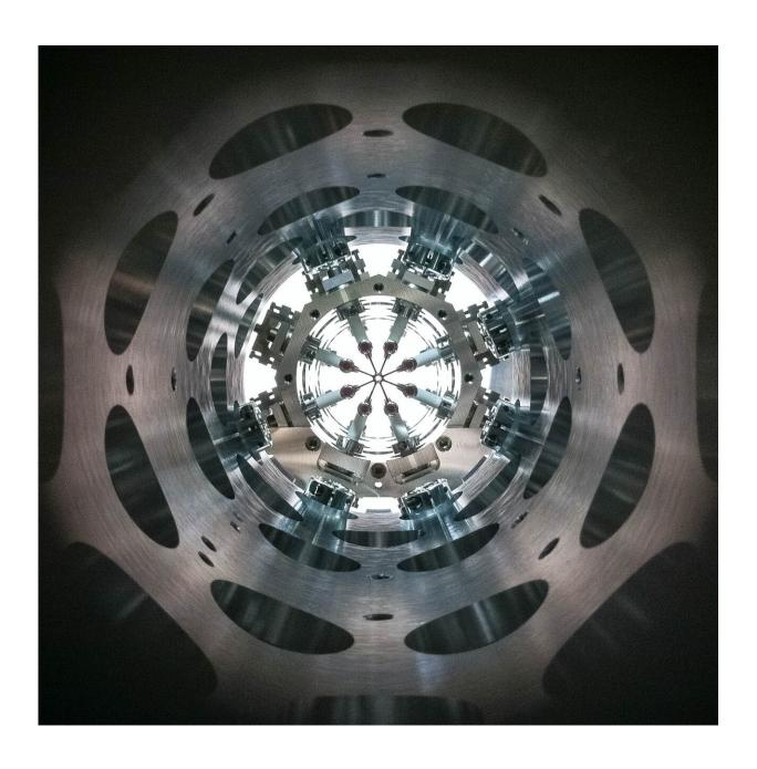
A lengthwise view inside the molecular trap: a series of high-voltage rings
