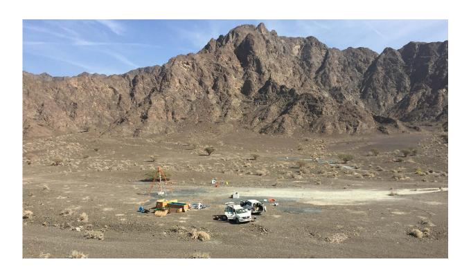
Researchers installed a packer system near Ibra, Oman, in January 2019 to study microbial communities in deep aquifers. The tripod installed at one well of a multiborehole observatory was used to suspend the packer assembly downhole. Credit: Nothaft et al.
