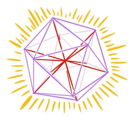
In a regular icosahedron (purple), six main interior diagonals (red lines) make equal angles with each other. Credit: Zilin Jiang
