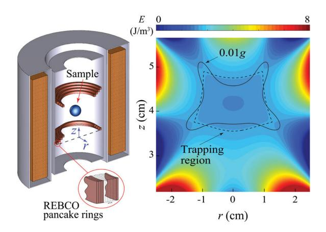
Left: A schematic of the magnet system designed by Sanavandi and Guo. Right: Contour plot of the trapping energy of a water sample placed in the proposed magnet, which shows the size and the shape of the region where the gravity is one percent of the Earth's gravity. Credit: Wei Guo/FAMU-FSU College of Engineering
