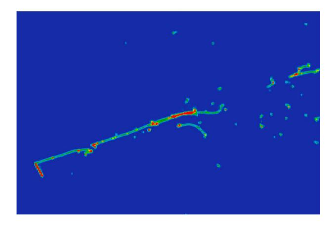
This approximately 70-centimeter-wide image depicts a MicroBooNE electron neutrino event, with an electron shower (straight line and dots bottom left to top right) and a proton track (short red line at bottom left). MIT researchers have been using the MicroBooNE experiment at Fermilab to uncover new secrets behind neutrinos. Credit: MicroBooNE Collaboration.
