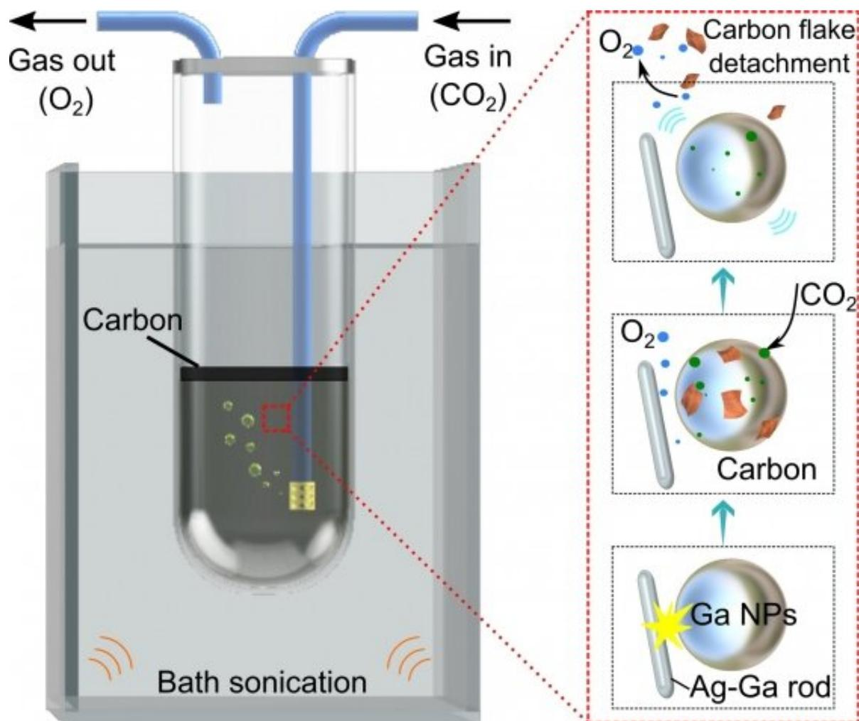
UNSW researchers have helped show how carbon dioxide can be broken down cheaply and efficiently via a process that dissolves captured CO<sub>2</sub> gas into a solvent around nanoparticles of gallium. Credit: University of New South Wales
