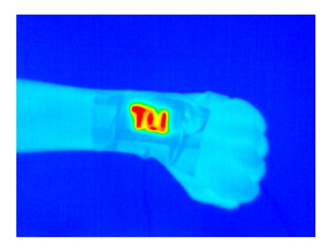
An electrically conductive and durable yarn was sewn onto fabric and became a wearable heater (high temperatures indicated by yellows and reds) when a safe voltage was applied. Credit: American Chemical Society
