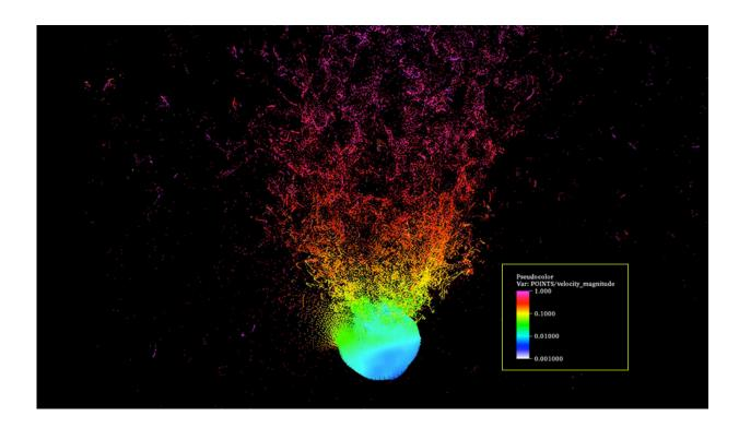
The hydro simulation in Spheral that provided the basis for the analysis: 1 Megaton at a few meters standoff distance from a 100-meter diameter asteroid (with Bennu shape). Colors denote velocities. The legend is cm/us, which is equivalent to 10 km/s. Credit: Lawrence Livermore National Laboratory
