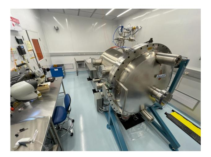
This is the SLAC thermal vacuum chamber which is used to do environmental testing on space-flight class laser systems. The ICESAT-2 and GEDI lidar mission made use of this chamber for qualification and risk reduction testing. The flight and engineering model Dragonfly Mass Spectrometer (DraMS) Lasers
