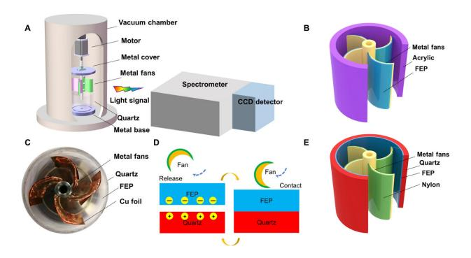
The schematic diagram of experiments. (A) CE parts in vacuum chamber and spectrometer. (B) Measurement mode A: FEP on fans and directly contact with quartz or acrylic. (C) Optical photograph of the CE parts. (D) The working principle of the measurement mode B. (E) Measurement mode B: FEP attached to quartz or acrylic with nylon, etc. on fans. Photo credit: Ding Li, Beijing Institute of Nanoenergy and Nanosystems, Chinese Academy of Sciences. Credit: Science Advances, doi: 10.1126/sciadv.abj0349
