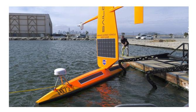
A type of autonomous marine robot called a Saildrone being deployed from Alameda, California. Credit: NASA / Jesse Carpenter
