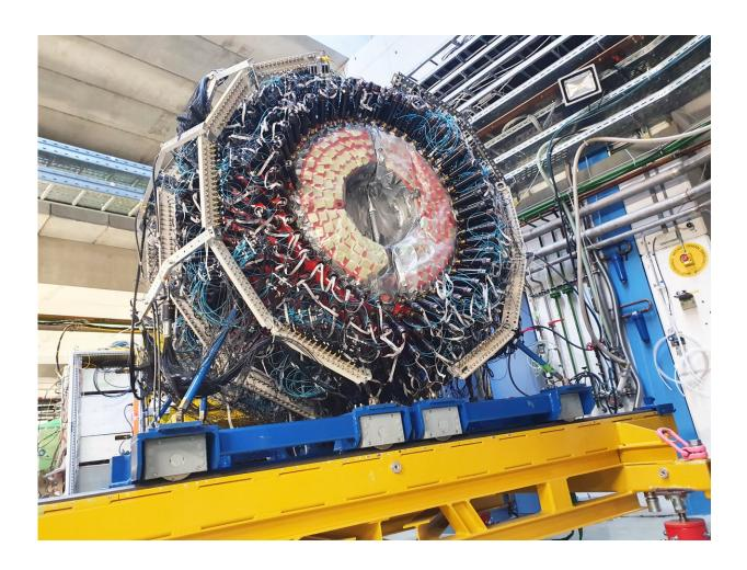
The gigantic WASA setup consists of scintillators and gaseous detectors that can detect charged and neutral particles. Credit: G. Otto, GSI/FAIR
