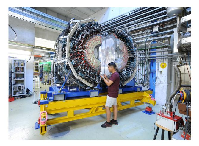
To make space for the superconducting solenoid magnet, the WASA detector can be opened in the middle. NUSTAR engineer Philipp Schwarz performs final work for the installation. Credit: G. Otto, GSI/FAIR
