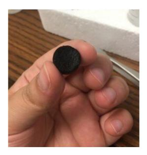
A hydrogel tablet developed by engineers at The University of Texas at Austin can purify a liter of river water in an hour or less. Credit: The University of Texas at Austin.
