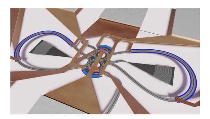
Three-dimensional rendering of the frequency translating add/drop filter showing two coupled active microring resonators, interferometric input/output waveguides, metal wires connected to electro-optic and thermo-optic phase shifters, and vertical grating couplers. Credit: Hayk Gevorgyan, Boston University
