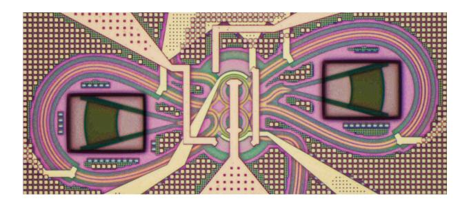
Optical microscope image of the second order frequency translating add/drop filter designed by the researchers in Boston University and implemented using IMEC's ISIPP50G active silicon photonics process. Credit: Hayk Gevorgyan
