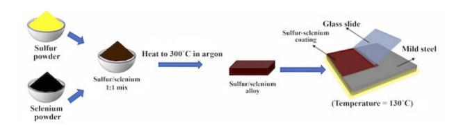
An illustration shows the simple process of combining powdered sulfur and selenium into a compound able to protect mild steel from the elements. Credit:
