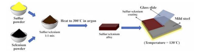
An illustration shows the simple process of combining powdered sulfur and selenium into a compound able to protect mild steel from the elements. Credit:
