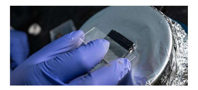
Rice University graduate student M.A.S.R. Saadi coats a compound of sulfur and selenium onto steel to test its ability to protect the surface from biotic and abiotic contaminants. Credit: Jeff Fitlow
