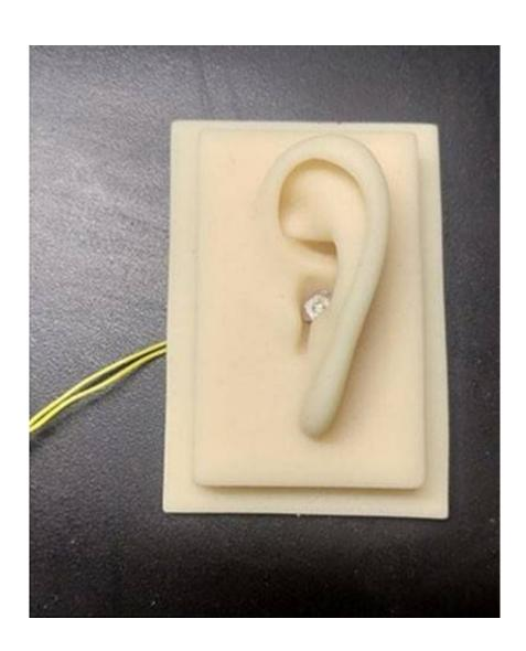
An electrically conductive membrane implanted inside a model ear simulates cochlear hairs by converting sound waves into electrical pulses; wiring connects the prototype to a device that collects the output current signal. Credit: *ACS Nano*
