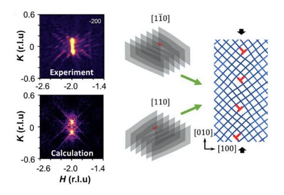
Irreversible, plastic deformation causes extended crystalline defects in the quantum material strontium titanate (SrTiO3) to organize into periodic structures, as revealed by neutron and x-ray scattering processes. These structures enhance electronic properties such as superconductivity. Credit: S. Hameed et al., University of Minnesota
