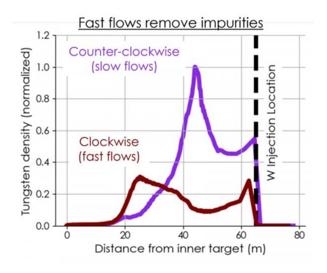
Simulation results showing tungsten density at the interface of the plasma's edge and core for both magnetic field directions. Fast flows that often occur in the clockwise magnetic field direction reduce the accumulation of tungsten impurities. Credit: Shawn Zamperini, UT-Knoxville.
