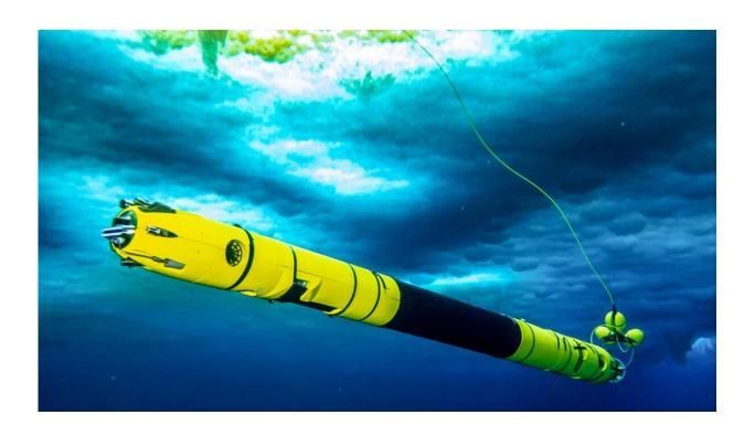
Icefin is a small robotic oceanographer that allows researchers to study ice and water around and beneath ice shelves – and develop the technology to explore other oceans in our solar system. Credit: Cornell University
