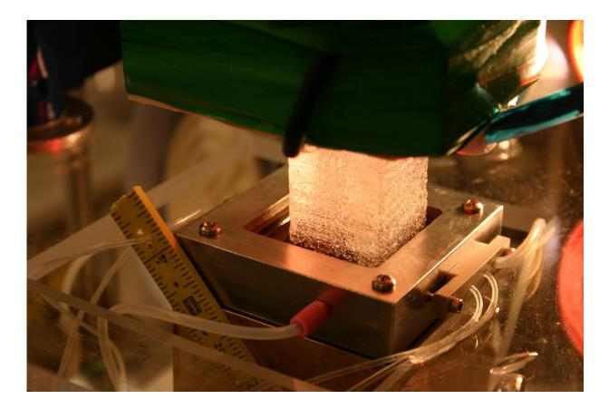
Measuring the chemistry in a longitudinal sample of an ice core on DRI's unique ice core analytical system. Credit: Joe McConnell/DRI
