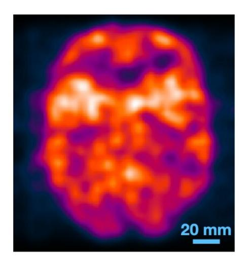
New ultrafast photon detectors allow for rapid processing of data from positron emission or X-ray scans without the need for tomography to reconstruct images. This image shows a brain phantom (model) scanned by positron emission using the new technology. Credit: Simon Cherry, UC Davis
