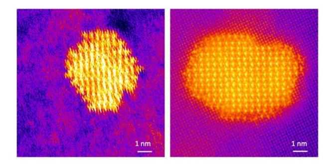
The transmission electron microscope image of an aluminum alloy on the left was distorted by intrusion of a magnetic field effect. Once the magnetic field was removed, the atomic-level clarity achieved is shown on the right. Credit: Libor Kovarik | Pacific Northwest National Laboratory
